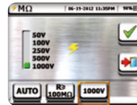
Selection of test voltage and minimum limit value
