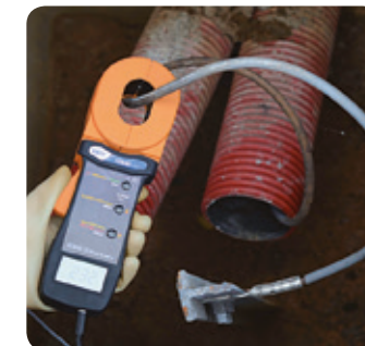
Measurement with clamp T2100
