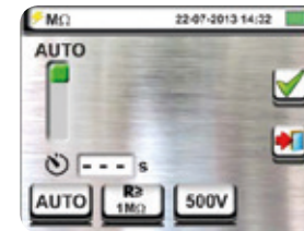
Selection of AUTO or TIMER measuring mode
